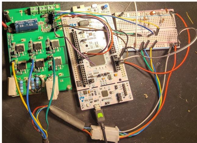
EV6532 with ST microcontroller and breadboard for pullup resistors.
